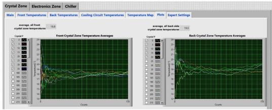
Screenshot of LabVIEW front panel for hardware interlock monitoring system program showing Plots tab
