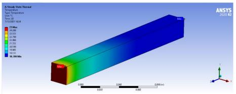
Central crystal of 3x3 cube of PbWO<sub>4</sub> with 25° C applied to its face
