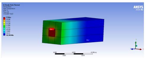
Thermal simulation of 3x3 cube of PbWO4 crystals with 25° C applied to face of central crystal
